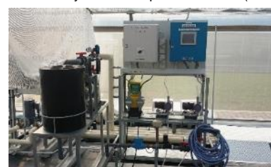
Smart fertiliser dispensing and self-filling water top up system
